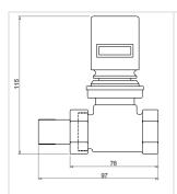
SRV2d two-way valve 3/4" with actuator
