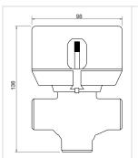
SRV3d three-way valve 3/4" with actuator Protection degree: IP44 Power supply: 200-240 V
